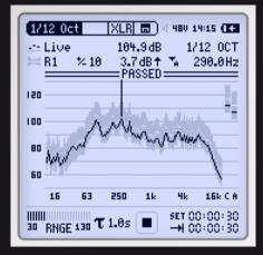
The Spectral Limits Option adds an RTA Analyzer with 1/6 and 1/12 octave spectral resolution and the Zoom-FFT. It extends the XL2 function range with trace capturing, relative curve display and comprehensive tolerance handling. The XL2 Analyzer compares spectral measurements against reference curves or a tolerance band including PASS/FAIL results.
