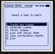
The Cinema Meter Option forms the dedicated solution for efficient calibration and repetitive verification of cinema loudspeaker systems according to SMPTE ST 202:2010 and RP 200:2012.
