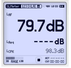
The XL2 provides a precise sound level meter for events and environmental noise monitoring. Numerous measurement variations are simultaneously available. Actual level, Lmin, Lmax, Leq may be measured in combination with frequency weighting A, C or Z and time weightings fast, slow and optional impulse. All results are simultaneously available.
