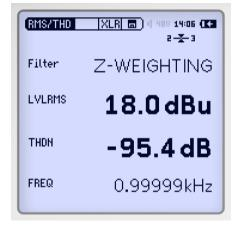
The XL2 with balanced XLR and unbalanced RCA inputs offers a comprehensive, high performance audio analyzer. It simultaneously measures balance, level, distortion (THD+N) and frequency.
